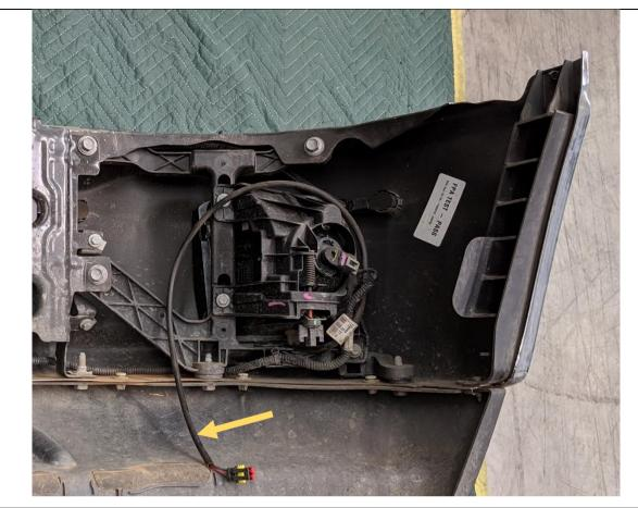
41. Remove the parker light plug by cutting off close to factory parker location for re-use on Offroad Animal bar.
