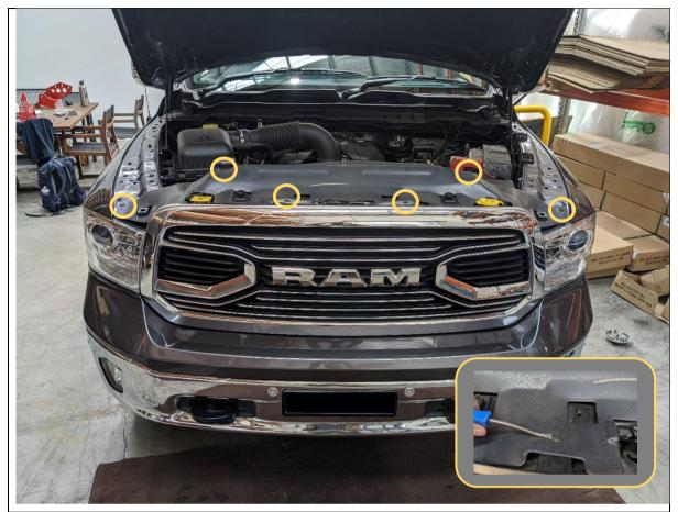
**NOTE:** The following steps show the removal of the split chrome type bumper as fitted to Laramie Models.
