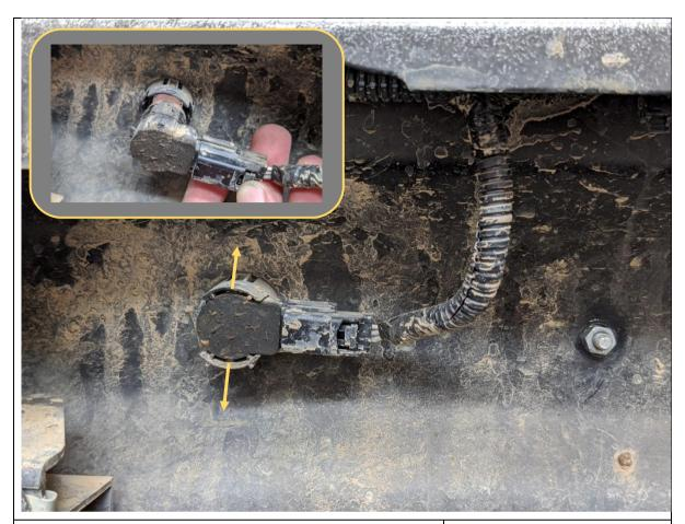
33. Remove parking sensors from housings. Gently pry apart housing, using a small flat screwdriver whilst pushing sensor through from the front side of the bar to release them.
