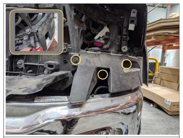
20. Remove the outer plastic bumper supports by removing the 3x 10mm hex screws securing it to the cross member.
