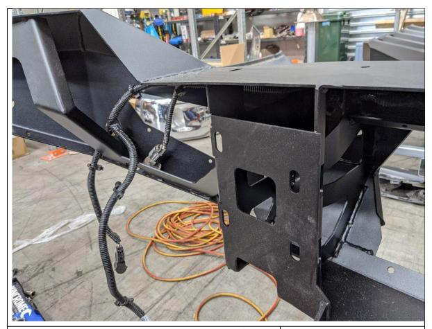
46. Pass wiring loom through bar uprights, starting from the left-hand side of the bar.
