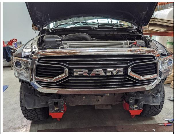
67. Re-fit grille to vehicle, replacing the 4x 10mm factory bolts.
