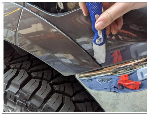
16. Using a Utility knife carefully cut the double-sided adhesive tape securing the wheel arch flare back to the bumper to guard joint in the body (see arrow in top left corner above).
